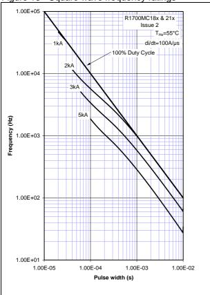
Figure 14 - Square wave frequency ratings
