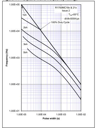
Figure 15 - Square wave frequency ratings
