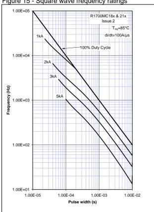
Figure 16 - Square wave frequency ratings
