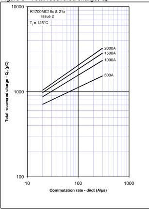
Figure 6 - Recovered charge, Q<sub>ra</sub> (50% chord)
