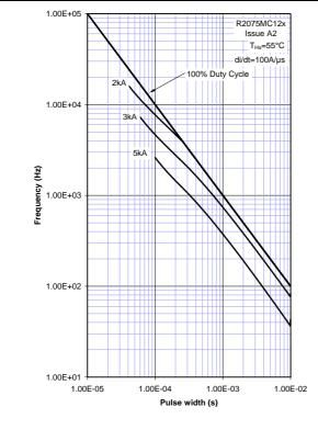
Figure 13 - Square wave frequency ratings
