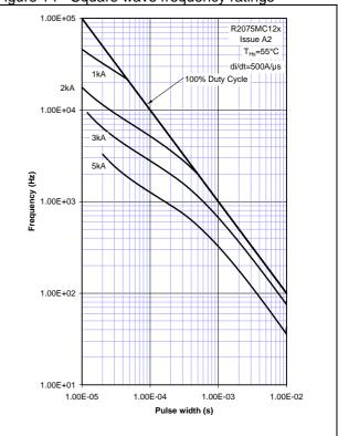
Figure 16 - Square wave frequency ratings
