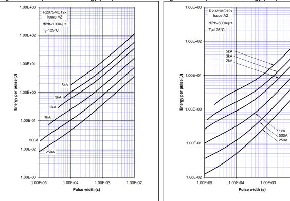
Figure 17 - Square wave energy per pulse
