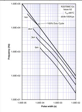
Figure 14 - Square wave frequency ratings
