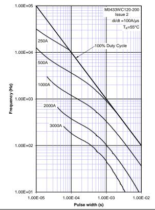
Figure 13 - Square wave frequency vs. pulse width
