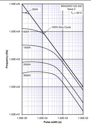
Figure 9 - Sine wave frequency vs. pulse width
