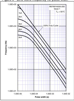
Figure 10 - Sine wave frequency vs. pulse width
