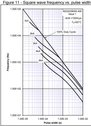
Figure 12 - Square wave frequency vs. pulse width
