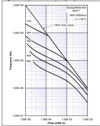
Figure 13 - Square wave frequency vs. pulse width
