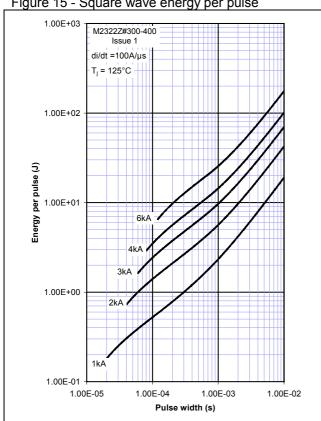
Figure 16 - Square wave energy per pulse
