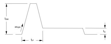
The magnitude of  $I_{GM}$  should be between five and ten times  $I_{GT}$ , which is shown on page 2. Its duration  $(t_{p1})$  should be 20µs or sufficient to allow the anode current to reach ten times  $I_L$ , whichever is greater. Otherwise, an increase in pulse current could be needed to supply the necessary charge to trigger. The 'back-porch' current  $I_G$  should remain flowing for the same duration as the anode current and have a magnitude in the order of 1.5 times  $I_{GT}$ .
