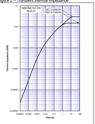
Figure 2 – Transient thermal impedance
