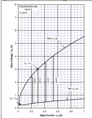
Figure 3 – Gate Characteristics – Power Curves
