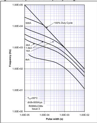
Figure 15 - Square wave frequency ratings
