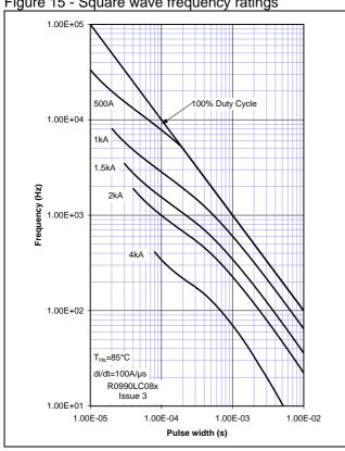
Figure 16 - Square wave frequency ratings
