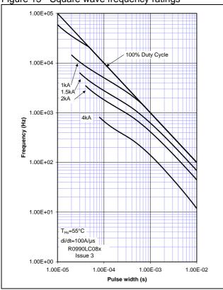
Figure 14 - Square wave frequency ratings
