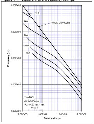
Figure 15 - Square wave frequency ratings
