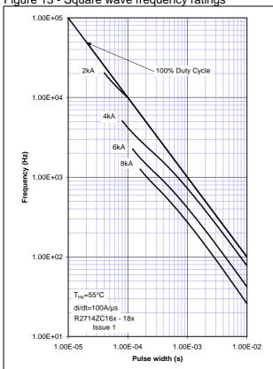
Figure 14 - Square wave frequency ratings
