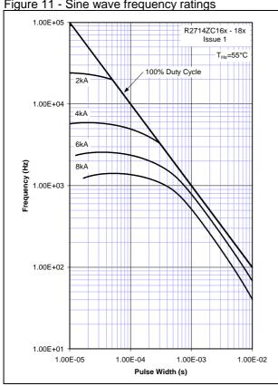
Figure 12 - Sine wave frequency ratings
