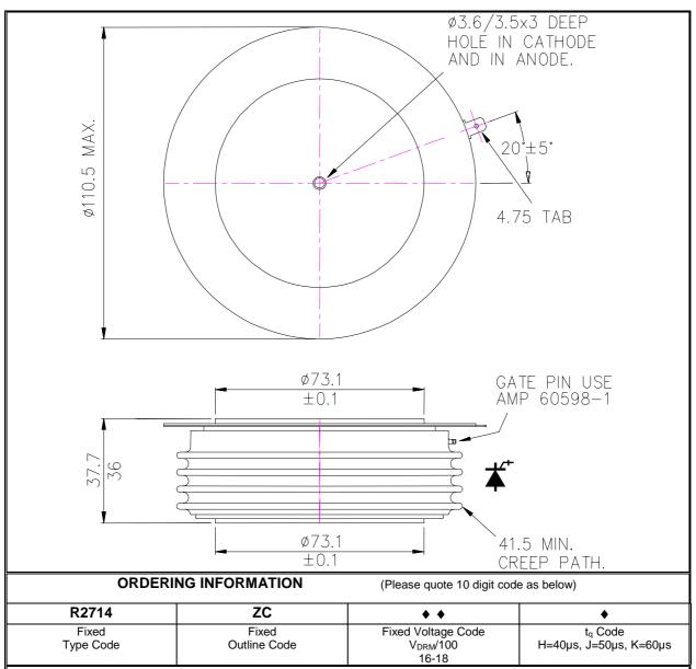
Typical order code: R2714ZC18K - 1800V V<sub>DRM</sub>, 60µs t<sub>q</sub>, 37.7mm clamp height capsule.
