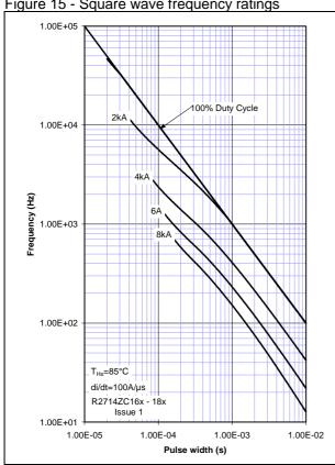
Figure 16 - Square wave frequency ratings
