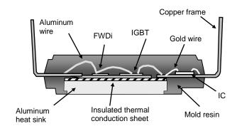
Fig.1-2 Internal cross-section structure
