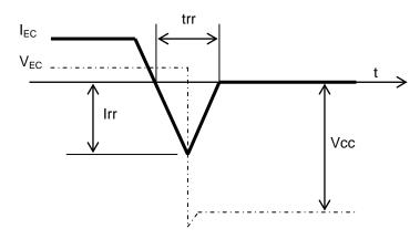
Fig.3-16 Ideal FWDi recovery characteristics curve
