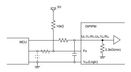
Fig.3-5 Control input connection
