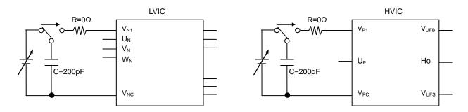
Fig.3-21 V<sub>N1</sub> terminal Surge Test circuit(V<sub>N1</sub> terminal)
