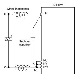
Fig.3-8 Recommended snubber circuit position
