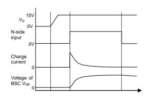
Fig.4-6 Example of waveform by one charging pulse
