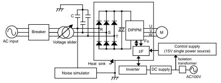
Fig.3-19 Noise withstand capability evaluation circuit
