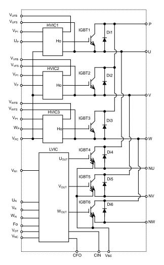
Fig.1-3 Internal circuit schematic
