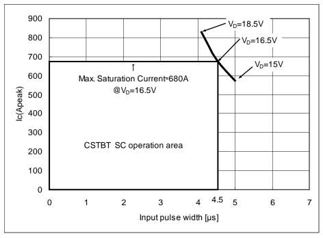
Fig.3-13 PS21A7A typical SCSOA curve
