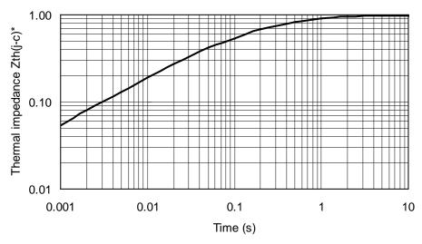
Fig.2-1 Typical transient thermal impedance
