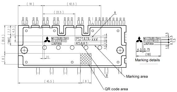
QR Code is registered trademark of DENSO WAVE INCORPORATED in JAPAN and other countries. Fig.2-17 Laser marking view
