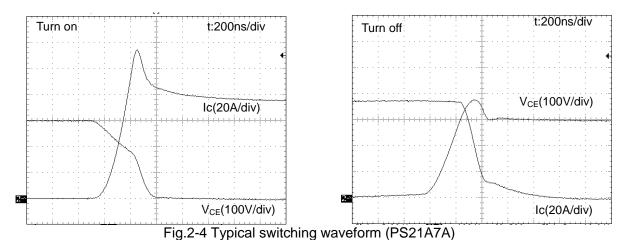
Conditions: V<sub>CC</sub>=300V, V<sub>D</sub>=V<sub>DB</sub>=15V, Tj=125°C, Ic=75A, Inductive load half-bridge circuit
