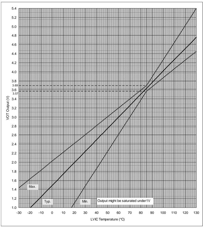
Fig.2-11 V<sub>OT</sub> output vs. LVIC temperature
