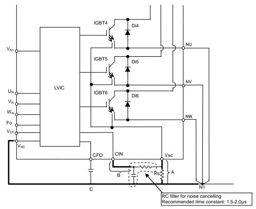
Fig.3-9 External protection circuit
