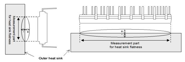
Fig.2-19 Measurement point of heat sink flatness
