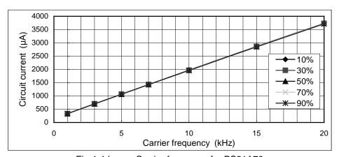
Fig.4-4  $I_{DB}$  vs. Carrier frequency for PS21A79
