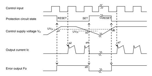
Fig.2-8 Timing chart of N-side UV protection
