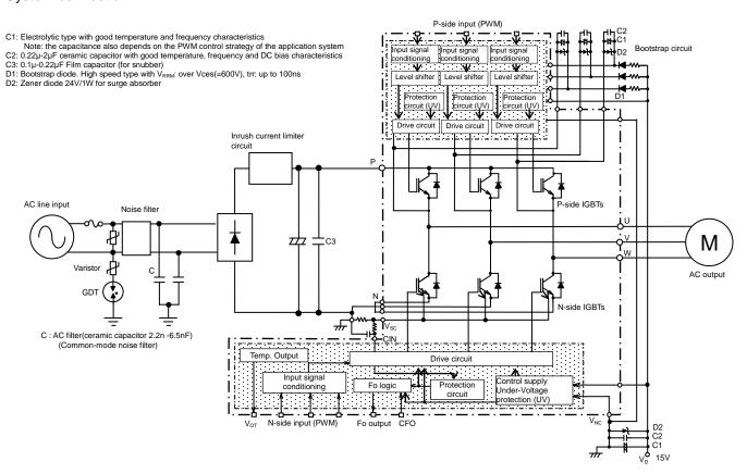
Fig.3-1 Application System block diagram
