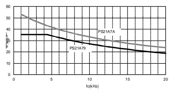
Fig.3-17 Effective current-carrier frequency characteristic
