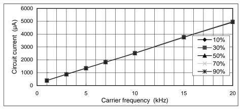
Fig.4-3 I<sub>DB</sub> vs. Carrier frequency for PS21A7A
