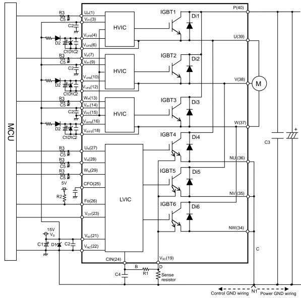
Fig.3-2 Interface circuit example (Direct coupling)
