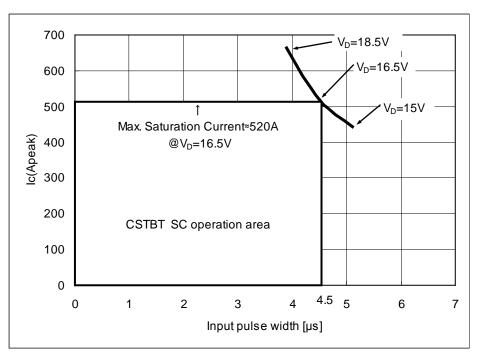
Fig.3-14 PS21A79 typical SCSOA curve
