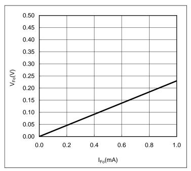
Fig.3-7 Fo terminal typical V-I characteristics (V<sub>D</sub>=15V, T<sub>i</sub>=25°C)
