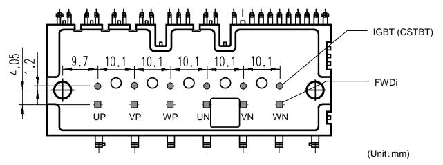
Fig.2-16 Power chip position
