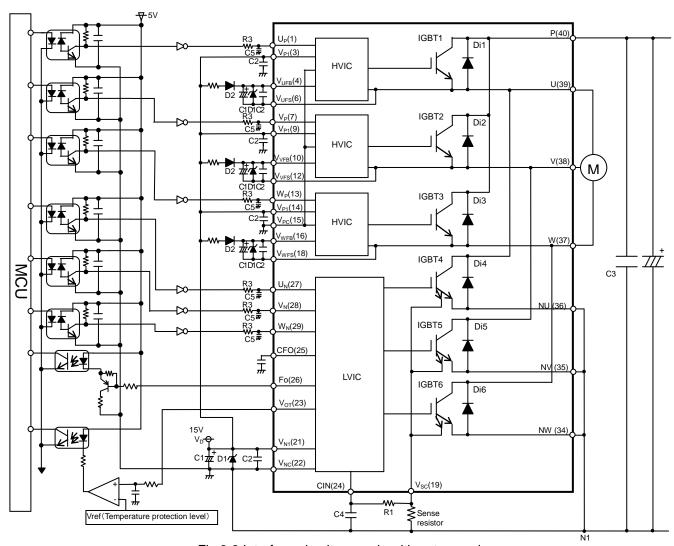
Fig.3-3 Interface circuit example with opto-coupler
