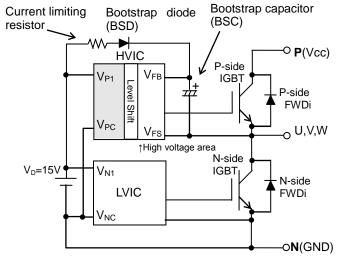
Fig.4-1 Bootstrap Circuit Diagram
