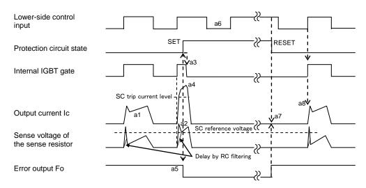
Fig.2-6 SC protection timing chart
