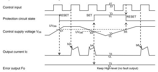
Fig.2-9 Timing Chart of P-side UV protection
