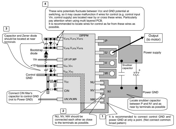
Fig.3-10 Precaution for wiring on PCB
