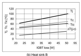
(a) Heat sink A (b) Heat Fig.2-12 IGBT loss vs. Tj, Tc, Tic(Ta=25°C, Typical)
