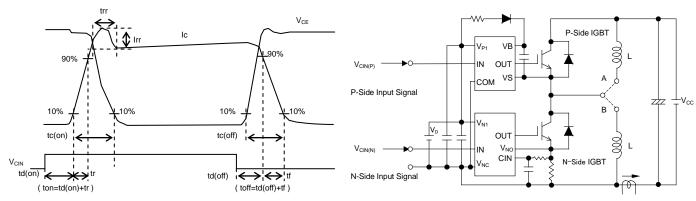
Fig.2-2 Switching time definition
