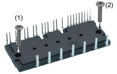
Fig.2-18 Recommended screw fastening order
