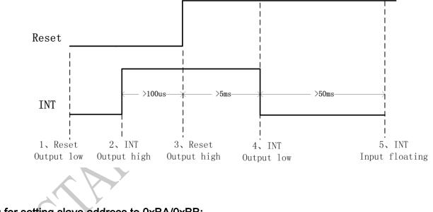
Timing for setting slave address to 0xBA/0xBB:
