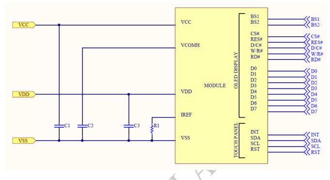
Recommended components: C1, C2 : 4.7uF/25V/0805 C3 : 1.0uF/16V/0603
