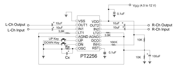
Note: Modifying the values of Rx and Cx affects the Oscillator Frequency of the IC. If the Fosc value is big, then the volume control change is fast. Likewise, if the Fosc value is small, the volume control change is slow. It is suggested that Rx=33K,  $Cx=2.2\mu$ F. The table for the Rx, Cx and Fosc values are given below.
