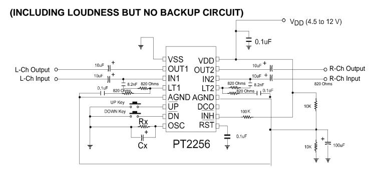
Note: Modifying the values of Rx and Cx affects the Oscillator Frequency of the IC. If the Fosc value is big, then the volume control change is fast. Likewise, if the Fosc value is small, the volume control change is slow. It is suggested that Rx=33K,  $Cx=2.2\mu F$ . The table for the Rx, Cx and Fosc values are given below.
