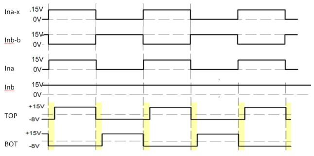
Input and output Signals with TOP-BOT configuration
