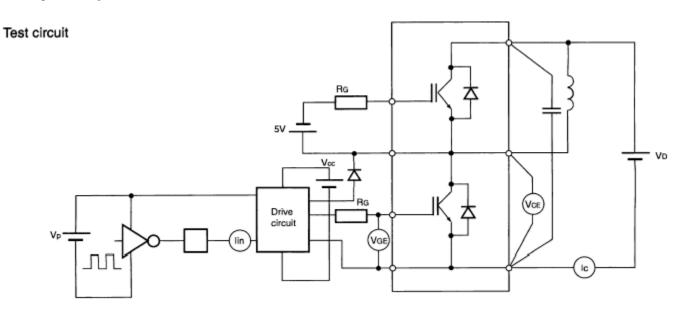
Operating conditions: Vcc=20V, Vd=600V, Ic=200A, IGBT module: 2MBI200U4B120, Rg=6 $\Omega$
