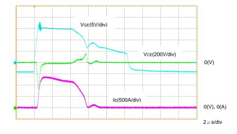
③Turn-on waveforms(At short circuit)
