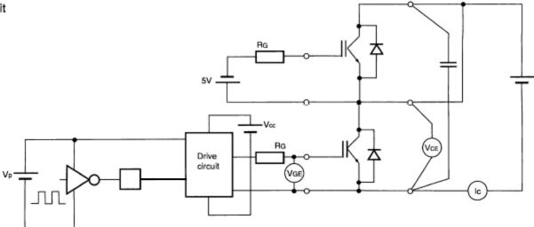
Operating conditions: Vcc=20V, Vd=800V , IGBT module: 2MBI200U4B120, Rg=6 $\Omega$
