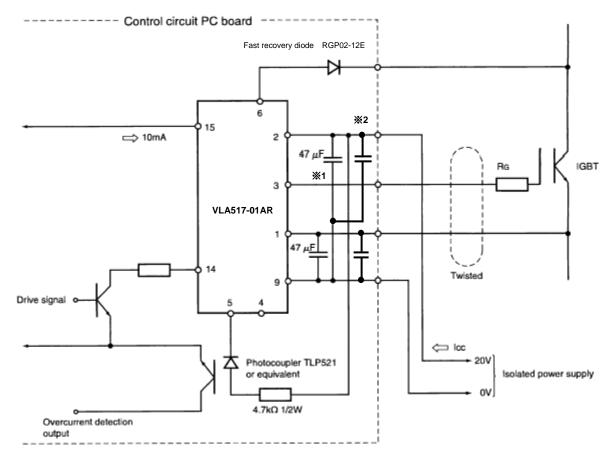
% The capacitor absorbs changes in the supply voltage caused by the power supply wiring impedance. It is not a power supply filter capacitor.
