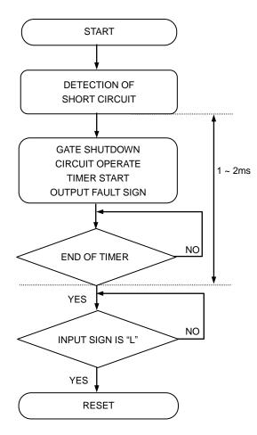
Note : "L" output voltage with protection circuit operating is about VEE + 2V.
