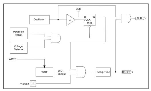
Fig. 4-7 Controller Reset Block Diagram
