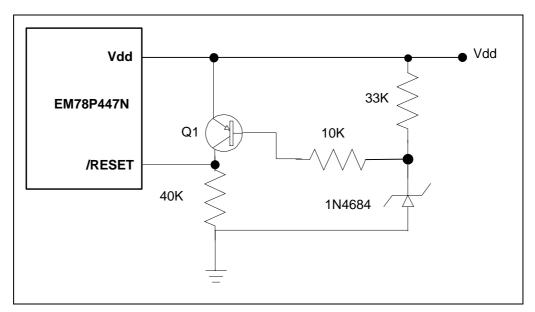
Fig.4-13 Residue Voltage Protection Circuit 1
