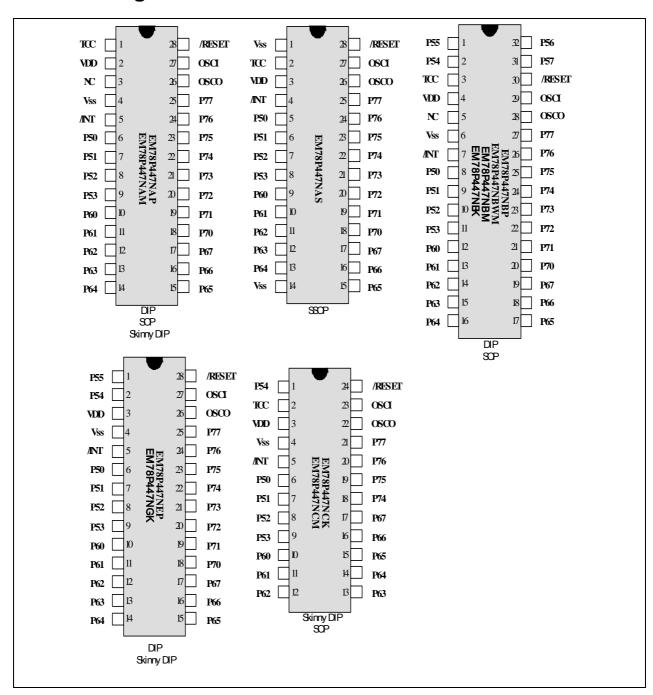
Fig. 3-1 Pin Assignment
