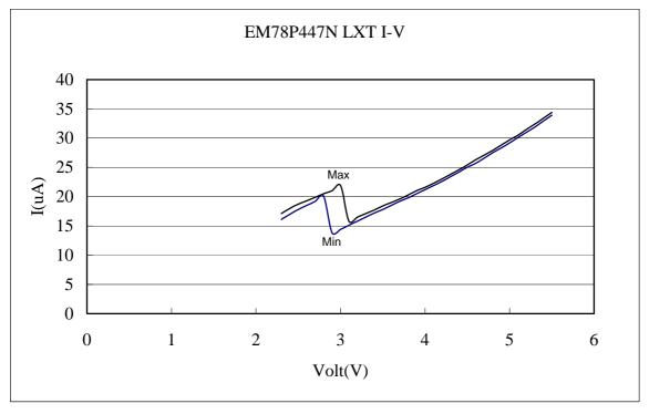
Fig. 6-20 EM78P447N I-V Curve Operating at 32.768 kHz
