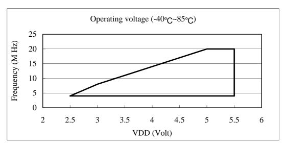
Fig. 6-18 Operating Voltage In Temperature Range from –40  $^{\circ}$ C to 85  $^{\circ}$ C
