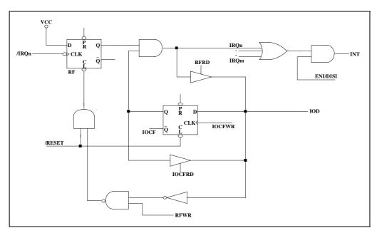
Fig. 4-8 Interrupt Input Circuit
