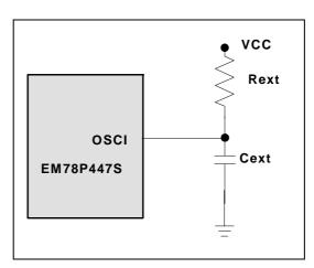
Fig. 4-11 External RC Oscillator Mode Circuit
