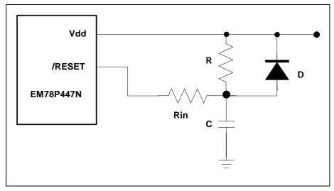
Fig. 4-12 External Power-Up Reset Circuit
