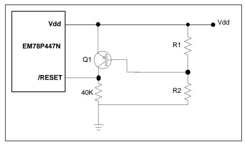
Fig.4-14 Residue Voltage Protection Circuit 2
