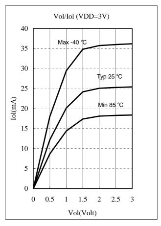
Fig. 6-6 Port 5, and Port 6 Vol vs. Iol, VDD=3V
