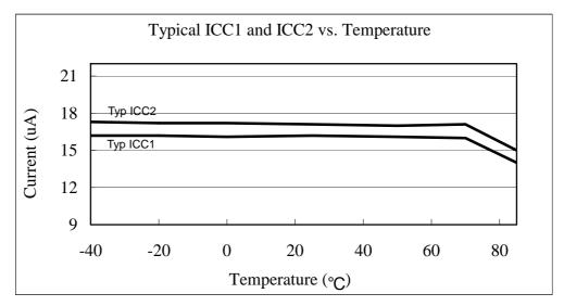
Fig. 6-12 Typical Operating Current (ICC1 and ICC2) vs. Temperature
