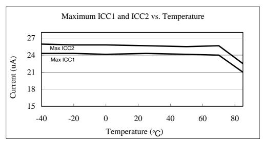
Fig. 6-13 Maximum Operating Current (ICC1 and ICC2) vs. Temperature
