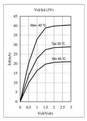
Fig. 6-8 Port 7 Vol vs. Iol, VDD=3V
