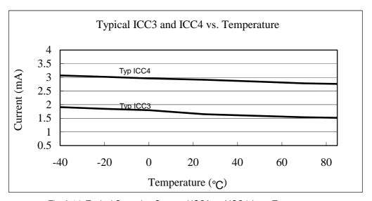
Fig. 6-14 Typical Operating Current ( ICC3 and ICC4 ) vs. Temperature
