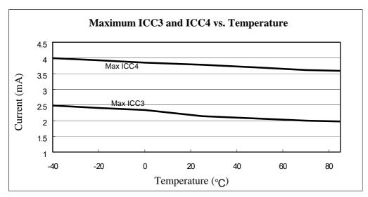
Fig. 6-15 Maximum Operating Current (ICC3 and ICC4) vs. Temperature
