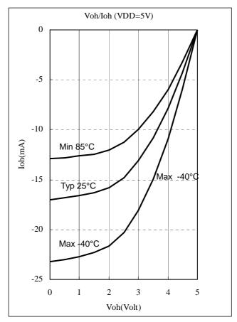
Fig. 6-3 Port 5, Port 6, and Port 7 Voh vs. Ioh, VDD=5V
