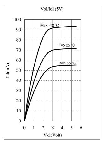
Fig. 6-7 Port 7 Vol vs. Iol, VDD=5V
