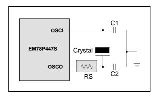
Fig. 4-10 Crystal/Resonator Circuit
