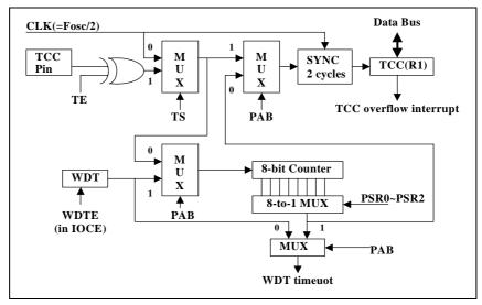
Fig. 4-5 TCC and WDT Block Diagram
