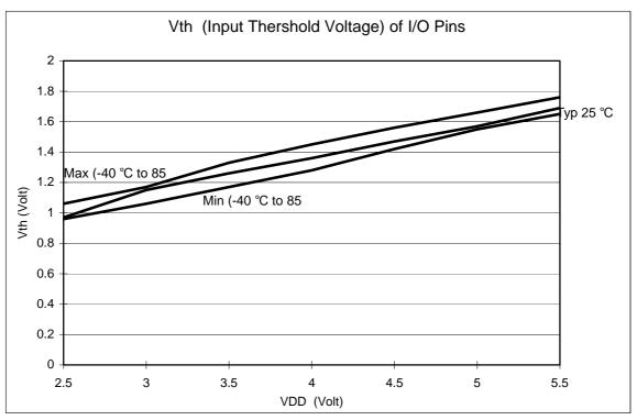
Fig. 6-2 Vth (Threshold Voltage) of P60~P67, P70~P77 vs. VDD
