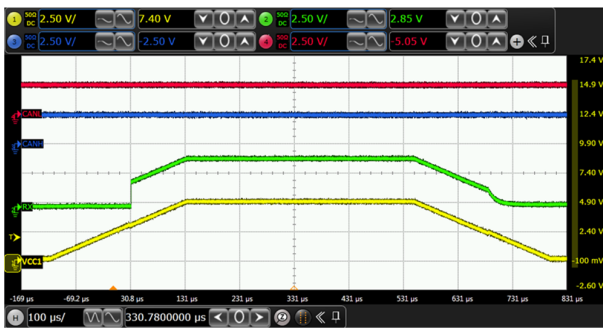
Figure 6-11. V_{OD(DOM)} Over V_{CC}
