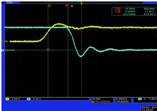
Figure 22. Propagation Delays with 1.8 nF Load
