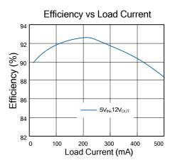
Figure 2. Efficiency vs Load Current
