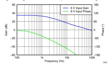
Figure 8-11. SEPIC Power Stage Gain and Phase
