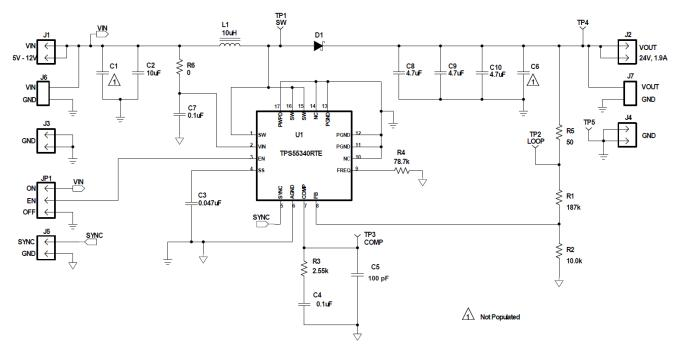
Figure 8-1. Boost Converter Application Schematic
