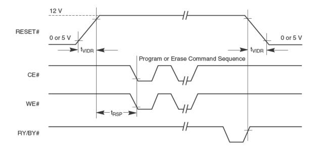
Figure 18. Temporary Sector Unprotect Timing Diagram
