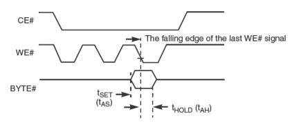
**Note:** Refer to the Erase/Program Operations table for  $t_{AS}$  and  $t_{AH}$  specifications.
