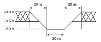
Figure 6. Maximum Negative Overshoot Waveform
