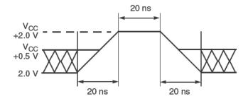
Figure 7. Maximum Positive Overshoot Waveform
