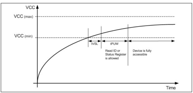
Figure 33a. Power-up Timing and Voltage Levels
