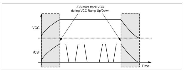
Figure 33b. Power-up, Power-Down Requirement
