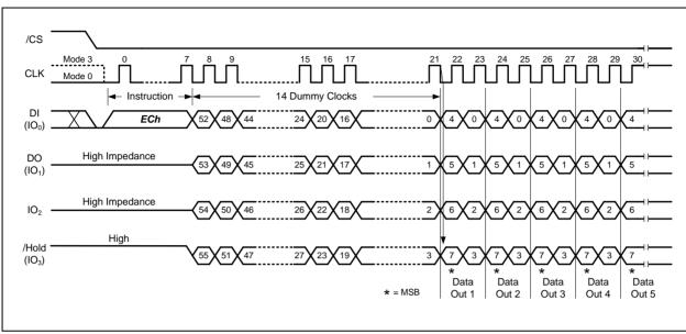
Figure 29b. Fast Read Quad I/O with 4-Byte Address Instruction (Continuous Read Mode, BUF=0)
