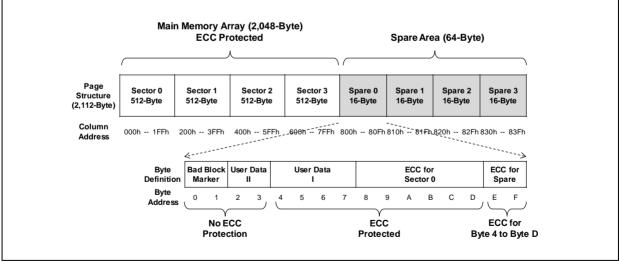
Figure 2. W25N512GV Flash Memory Architecture and Addressing
