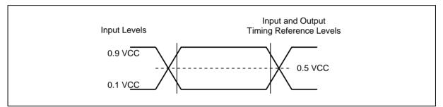
Figure 34. AC Measurement I/O Waveform
