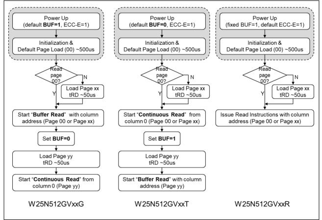
Figure 3. W25N512GV Flash Memory Operation Diagram
